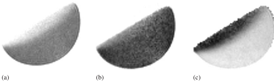
FIG. 8. Mustard seeds flowing in a drum. (a) Only the zeroth moment is nulled, and the image shows significant signal attenuation (visible as the lighter shades in the sliding layer) due to the velocity distribution in each pixel and higher-order contributions. (b) The first moment is nulled. There is no signal loss due to the velocity distribution; the remaining signal attenuation reflects velocity fluctuation and diffusion in the presence of background gradients. (c) Diffusion image. The darkness of the image is proportional to the diffusion coefficient D perpendicular to the plane of the image, calculated from signal attenuation in the presence of a gradient applied along the cylinder axis. All images were acquired at a ^1\text{H} frequency of 80 MHz. Reprinted with permission from Fukushima (1999), copyright 1999, Annual Reviews www.annualreviews.org .
